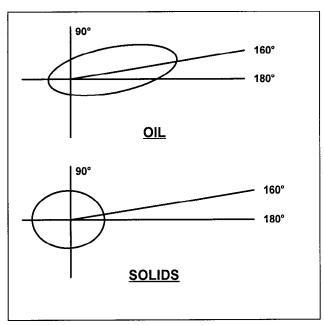
favor the 160° position. So with equal amounts of oil and solids in the water, the length of the vector at 160° for oil would be very large compared to the length of the vector from an equal amount of solids, therefore the solids will have little effect. With twice as much solids as oil, the solid circle would still be smaller, at the 160° position, and there is still no problem. Only when the solid's content exceeds four times the oil content do we have inaccuracy in our measurements.
