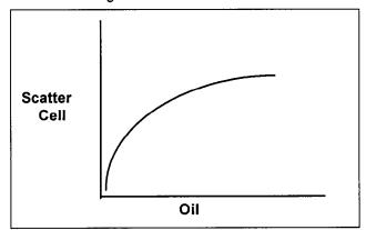
zero with no oil present [due to the occluding rod] and it increases with the oil content. Clearly, the light increases in a nonlinear way.
